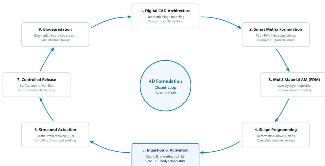
Figure 4. Working principle of a 4D-printed pharmaceutical system
