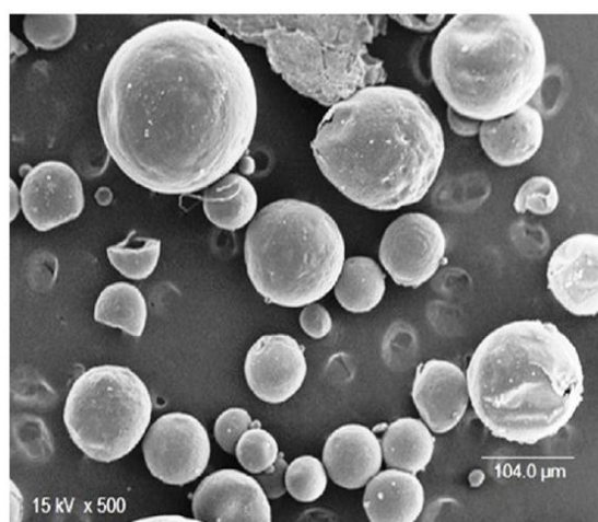
Figure 3. SEM of Floating Hollow Microspheres of Dexlansoprazole
