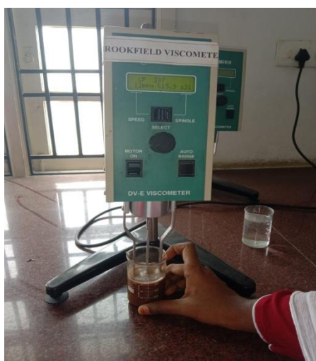
Figure 2 Measurement of Viscosity of Herbal shampoo by Brookfield Viscometer
