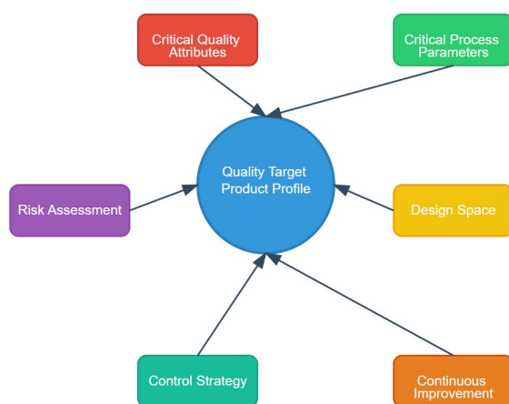
Figure 2. Quality by Design for Tablet Coating
