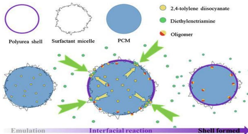
Figure 3 Interfacial reaction
