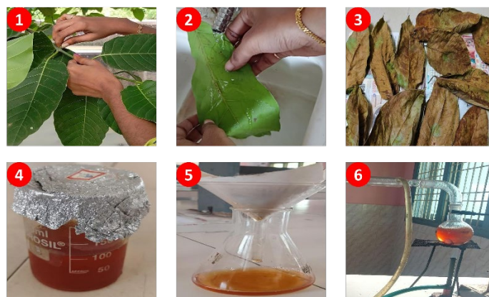
Figure 2. Extraction Process of leaves of N. cadamba 1. Collection 2. Washing 3. Drying 4. Maceration 5. Filtration 6. Distillation
