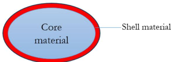
**Figure 1.** Core and Shell material of microparticles
