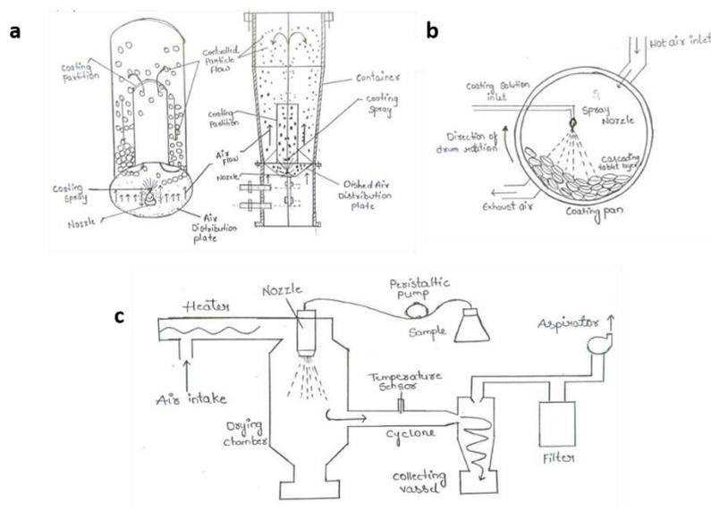
**Figure 2.** a. Air suspension process b. Pan coating c. Spray drying
